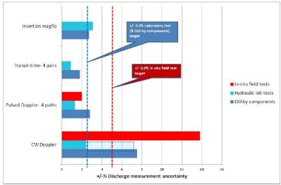
Discharge measurement uncertainty comparison for 0.5m/s velocity
